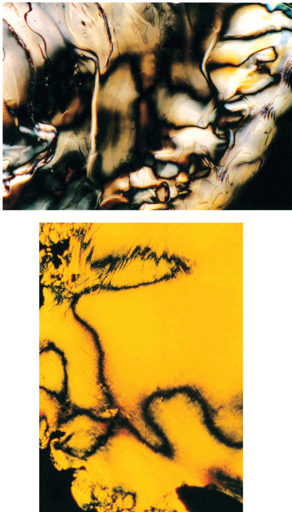
Figure 4. Optical textures of polymer 5a at 175 °C (top) and polymer 5b at 195 °C (bottom).
